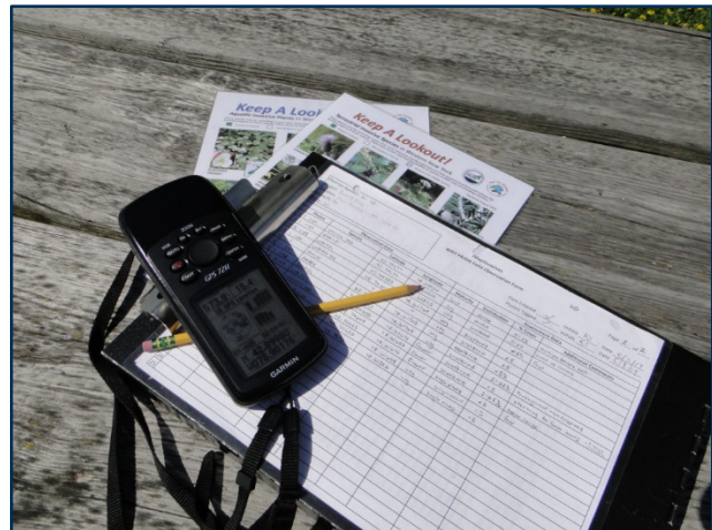
Tools of the trade, WNY PRISM uses handheld GPS units and data and identification sheets to collect iMap data in the field.
